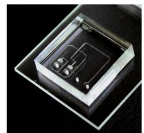
Figure 3: A Pico-Gen™ biochip for picodroplet generation.
